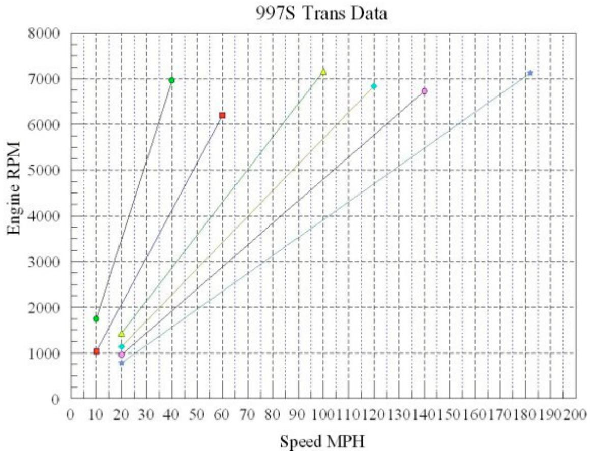
Figure No. 3 Engine Rpm and Vehicle Speed for Each Transmission Gear Ratio for a Given differential Ratio ( in this case 3.44:1 ).
