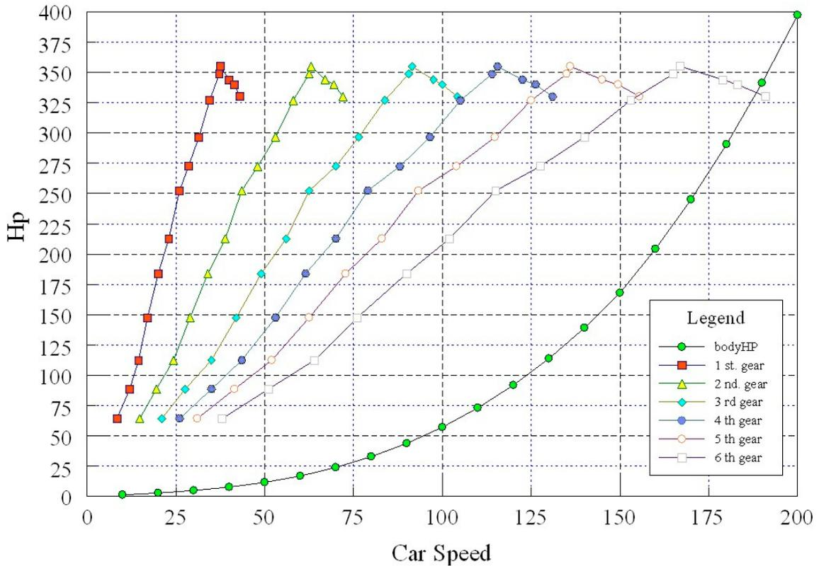
Figure No. 4 Hp Available in Each Gear and Hp to Drive the Car at Any Speed
