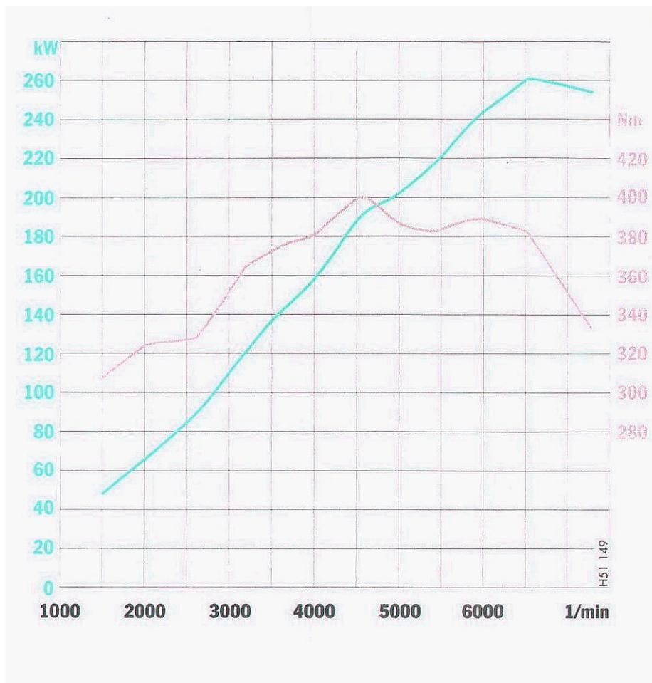
Figure no. 2 Engine Hp and Torque from the Owners Manual
